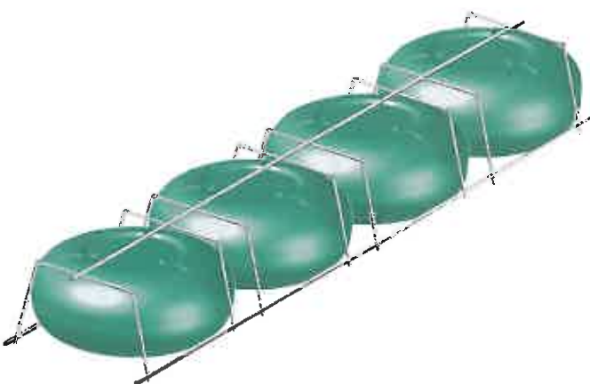
Fig. 16. Cage module with flattened void formers
