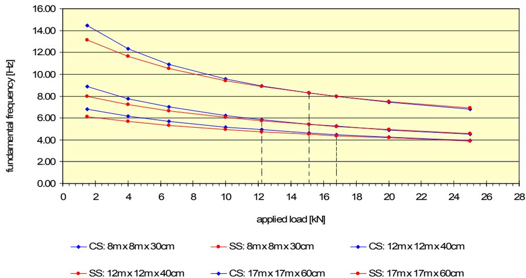
**Figure 4.7** Accuracy of ‘critical’ load for continuous slab
