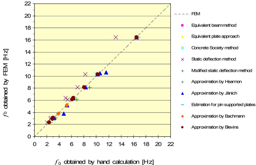
**Figure 3.2** Comparison of hand-calculated and computed frequencies
