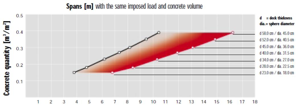
Figure C.1 Comparison of spans and concrete quantity
