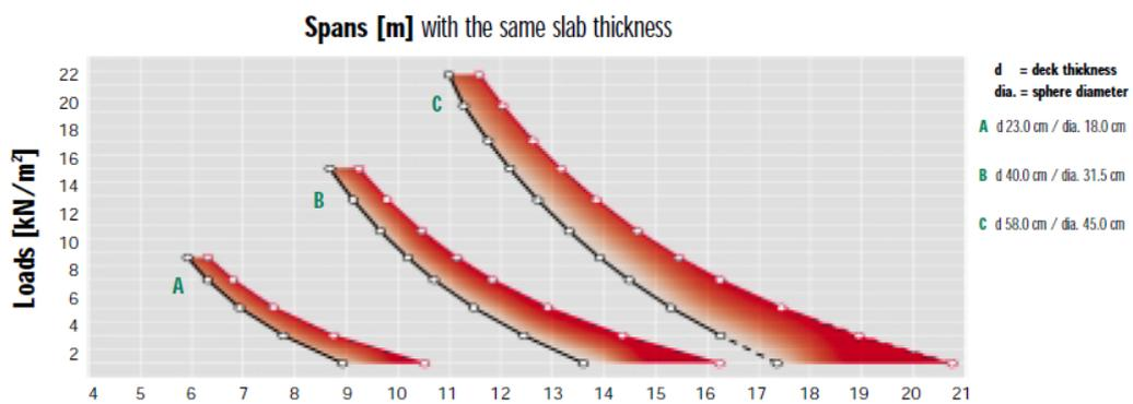
Figure C.2 Comparison of spans and loads
