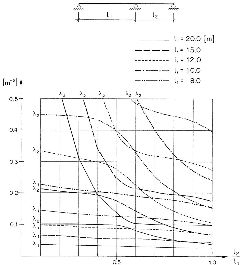
Figure 3.1 Frequency parameter for continuous slabs
