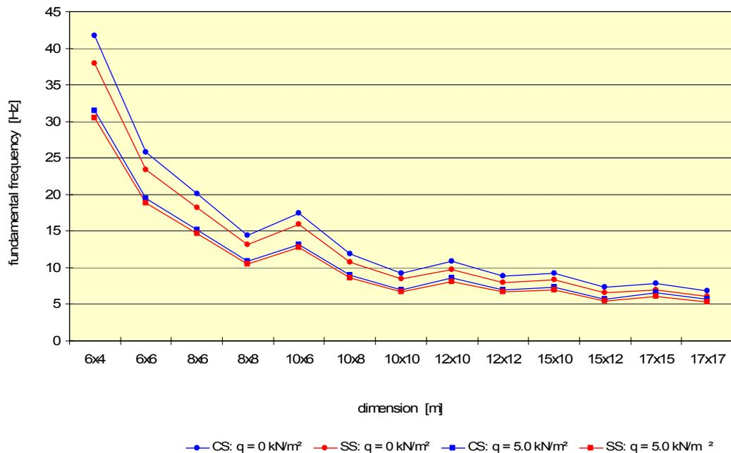
**Figure 4.4** Fundamental frequencies for a single span slab
