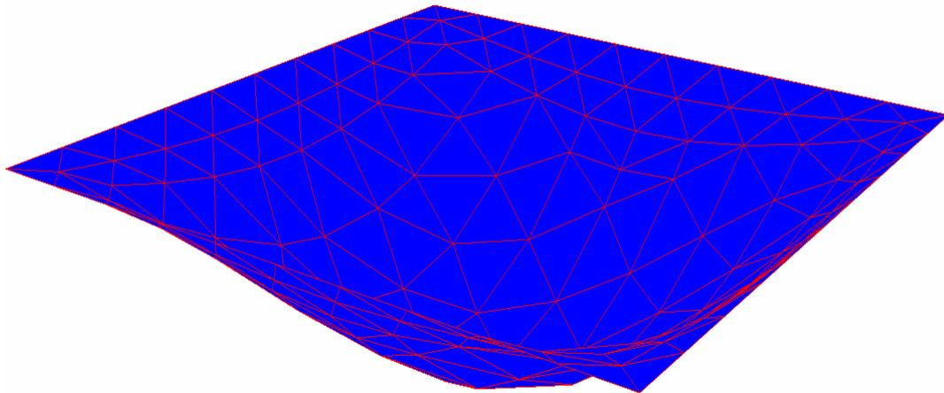
Fundamental frequency  $f_0$  : 7.135 Hz
