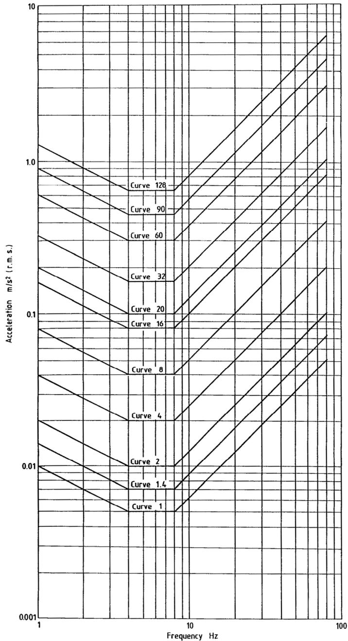
**Figure 2.2** BS 6472 (1992) Building vibration z-axis curves for acceleration (r.m.s.)
