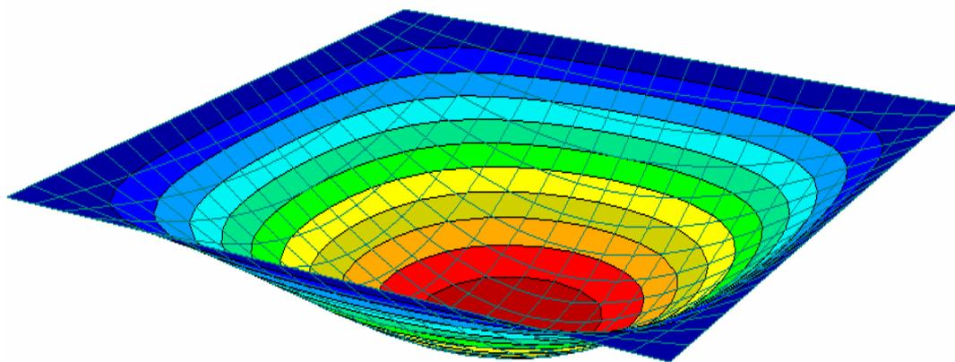
Fundamental frequency  $f_0$  : 7.148 Hz
